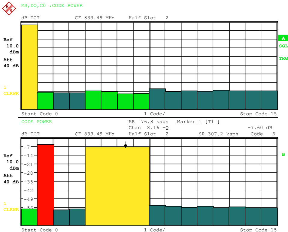
Fig. 18 CDP diagram in BitReverse order in Overview mode
